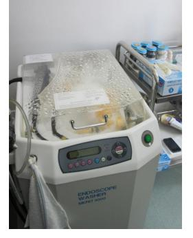
If the channels cannot be cleaned and disinfected in this machine, it might be better to stop working with it and go back to manual cleaning and disinfection – or buy a new real washer-disinfector.
